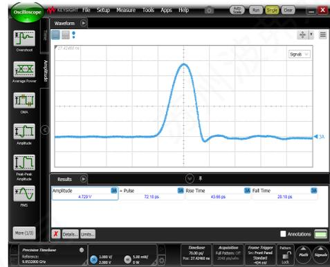
Output response: Pulse amplitude = 4.7 V<sub>pp</sub>, Rise time = 32 ps
