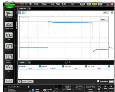
Output response: Pulse amplitude = 4.8 V<sub>pp</sub>, Rise time = 32 ps
