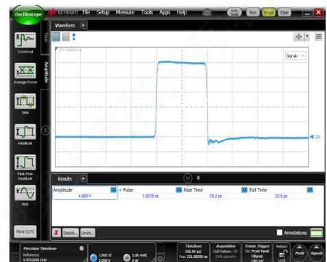
Output response: Pulse amplitude = 5 V<sub>pp</sub>, Rise time = 32 ps
