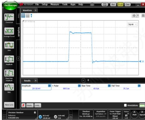
Input signal: Pulse amplitude = 0.25 V<sub>pp</sub>, Rise time = 32 ps
