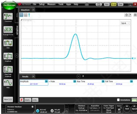
Input signal: Pulse amplitude = 0.22 V<sub>pp</sub>, Rise time = 24 ps
