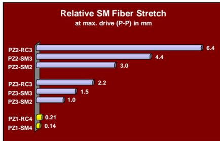
The **OPTIPHASE PZ1** is the high-speed member of our family of fiber stretchers. It is a fiber wound piezoelectric element for use in a wide range of optical interferometric measurement and sensing system applications. Typical uses include open loop demodulation, sensor simulation, variable optical delay, general purpose fiber interferometry and large angle modulation of interferometric phase.
