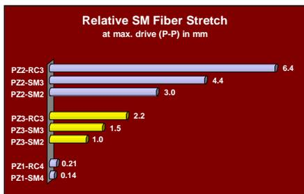
The *OPTIPHASE PZ3* is the mid-range member of our family of fiber stretchers. It is a fiber wound piezoelectric element for use in a wide range of optical interferometric measurement and sensing system applications. Typical uses include open loop demodulation, sensor simulation, variable optical delay, general purpose fiber interferometry and large angle modulation of interferometric phase.
